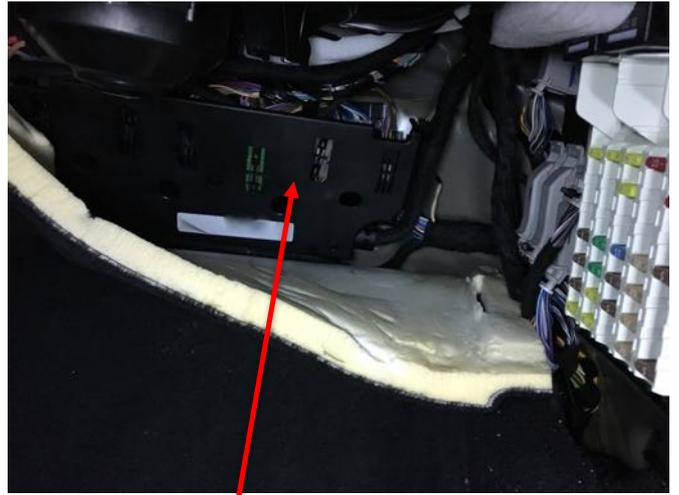
Plug cover with CAN wires
