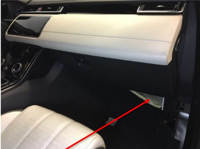
Connector with CAN wires
